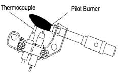
Figure 13 - Correct Pilot Flame Pattern
